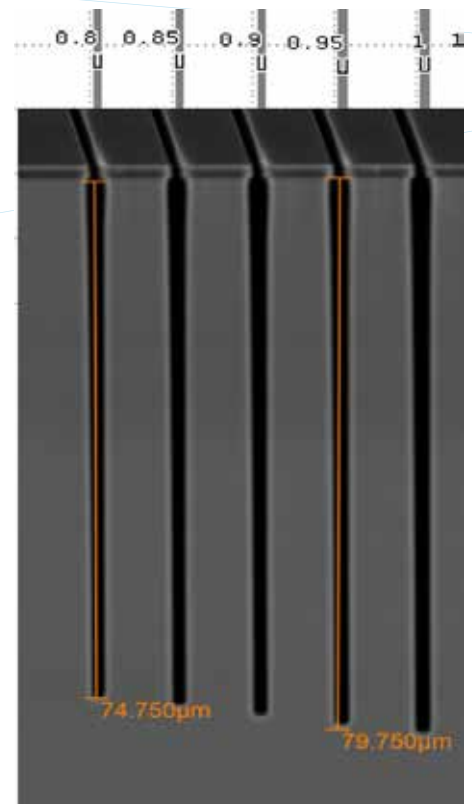
DRIE test structures with different gap widths showing Aspect Ratios of 80:1
